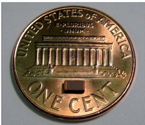
Fig. 9 One-cent magnetoelectric multilayer capacitor (Israel *et al.*): photograph, emphasizing size and cost (both M US\$0.01).<sup>17a</sup>
