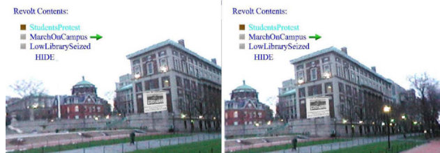
Figure 6. World-stabilized image snippet is fixed at its world location as user looks around.
