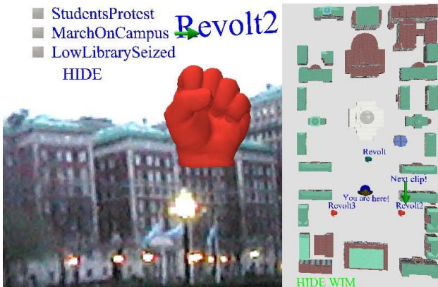
Figure 7. Screen-stabilized world in miniature indicates user’s current location and the Revolt2 icon containing the linked clip. The user has turned toward the Revolt2 icon, but hasn’t selected it, so the clip menu for Revolt is still displayed.
