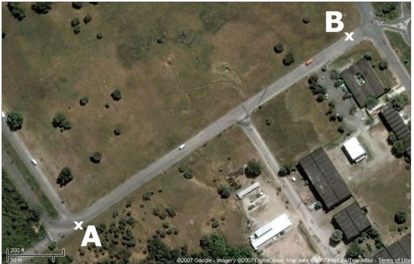
Figure 1. Satellite view of the 400-m-long street used for the experiment. Vehicles have two different start points (noted A and B); these points are far away enough so that nodes are not within the communication range of each other.
