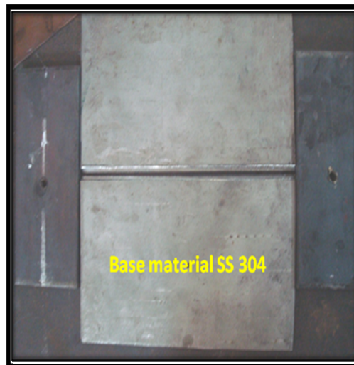
Figure 2 Specimen is tapered for weld strength.
