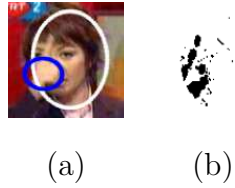
Figure 4.3. Tracking during hand-face occlusion: (a) Tracking result when the hand is in front of the face. (b) The movement of the face pixels
