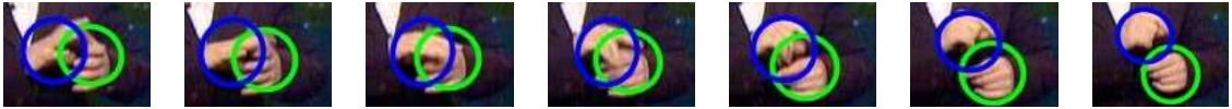
Figure 4.2. Tracking during hand-hand occlusion. Blue and green ellipses show the estimates for the right and left hands
