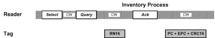
Fig. 5. “Select” command in the EPCglobal UHF Class 1 Generation 2 protocol [10]. A particular tag population is selected before the inventory process is initiated with the “query” command.
