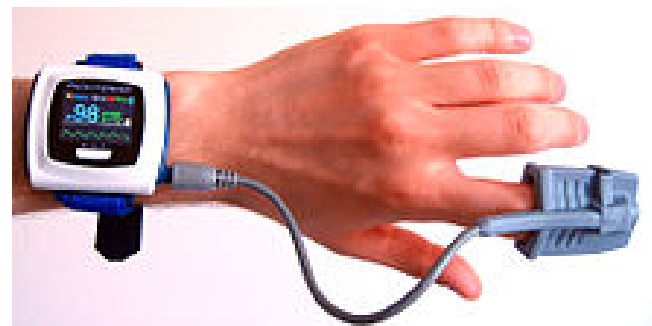
Fig.4: Pulse Oxy meter and its principle of operation
