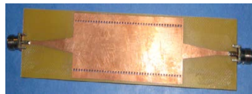
Fig. 3 A Photograph of the manufactured SIW- microstrip line with tapered transitions
