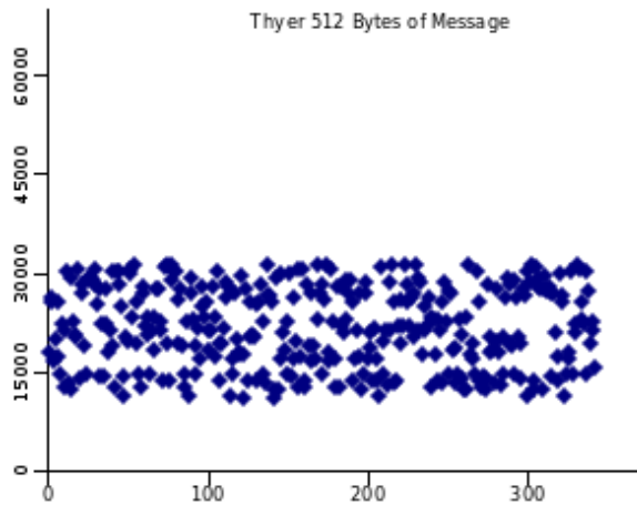
Fig. 2 The randomness distribution of the DNS ID taken from Tyher CC when embedded 512 bytes of a message
