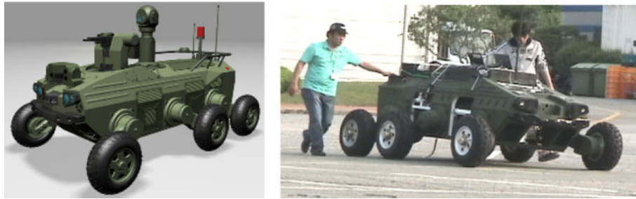
Fig. 1 Robotic vehicle with articulated suspension (RVAS)
