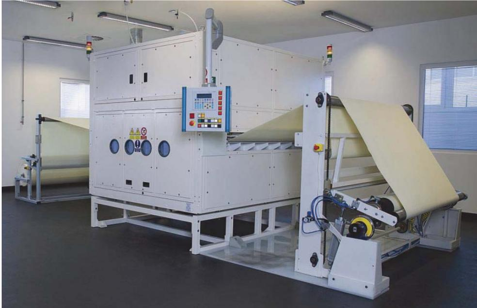
Fig. 10. Nozzle-less production electrospinning line (Nanospider™).
