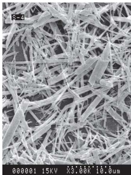
Fig. 11. MoO<sub>3</sub> morphology of precursor of 26% AHM at acidity coefficient 22 (180°C for 40h).
