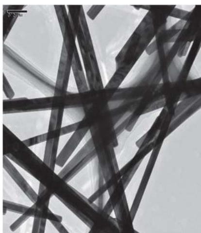
Fig. 13. Typical image of MoO<sub>3</sub> nano fibers characterized by HRTEM.
