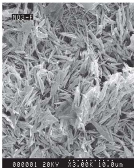
Fig. 8. MoO<sub>3</sub> morphology synthesized at 1.0 moles ratio of CTAB with AHM under 180°C for 40h.
