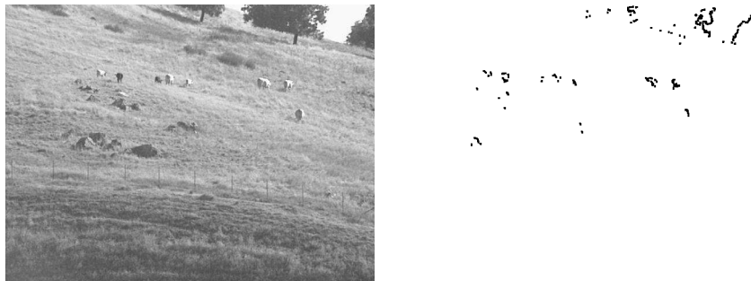
Figure 3: Edge detection in a scene outside the IBM Almaden Research Center. On the left is the raw image and on the right are the edges detected with a brightness threshold of 75.
