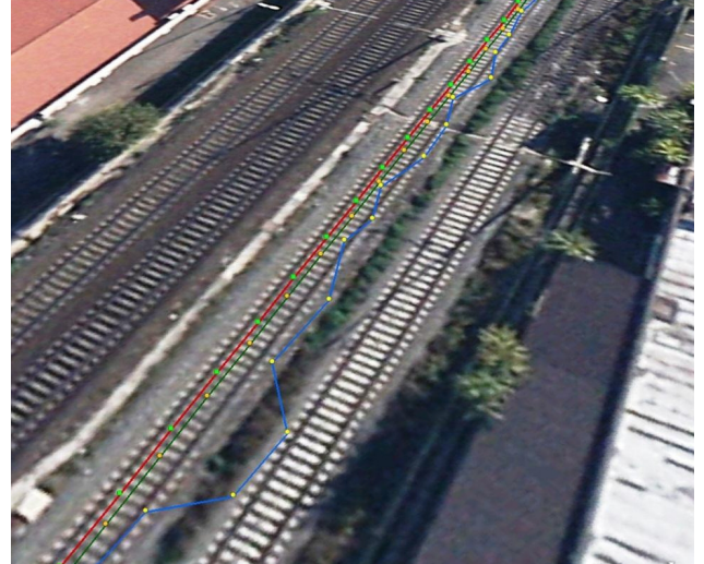
Figure 2. Detail of the Roma-Salerno measurement campaign: RTK unconstrained estimate (green-line) and code based Differential GNSS (blue line) versus ground truth (red line).
