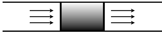
FIG. 2 Color online. Schematic of an experiment measuring mass flow through a supersolid. Superfluid liquid flows across the central section filled with supersolid, of the same substance. The setup as shown can work only at the melting pressure. In the case of ^4\text{He} , modifications involving Vycor segments and temperature gradients allow one to extended measurements to higher pressures (Ray and Hallock, 2008).
