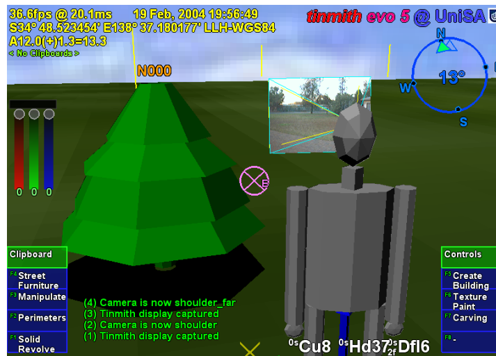
Figure 4-21 VR view of final surface of revolution tree as a solid shape
