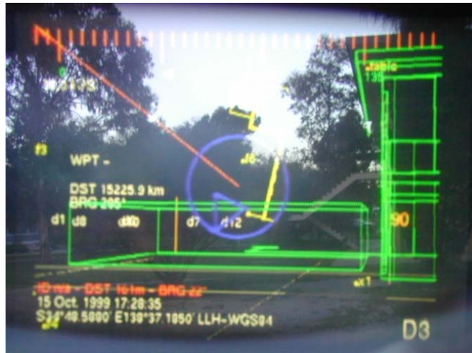
Figure A-7 3D wireframe overlay of building, with small extension made to the left
