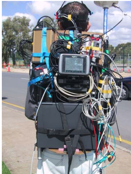
Figure 7-2 Rear view of previous backpack design, showing tangled mess of cabling
