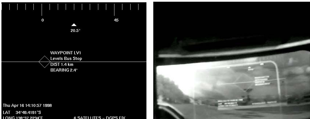
Figure A-3 Screen shots of Map-in-the-Hat indicating a waypoint on the display
