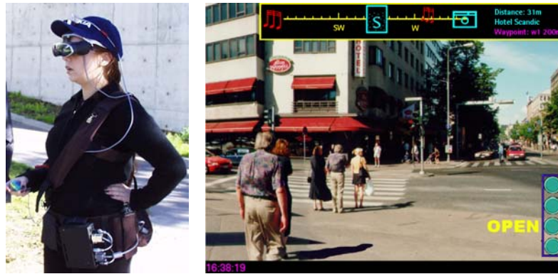
Figure 2-12 Context Compass provides navigational instructions via AR overlays (Images courtesy of Riku Suomela – Nokia Research Lab)
