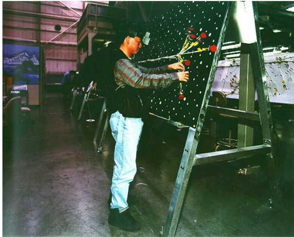
Figure 2-5 Worker using an AR system to assist with wire looming in aircraft assembly (Image courtesy of David Mizell – Boeing Company)
