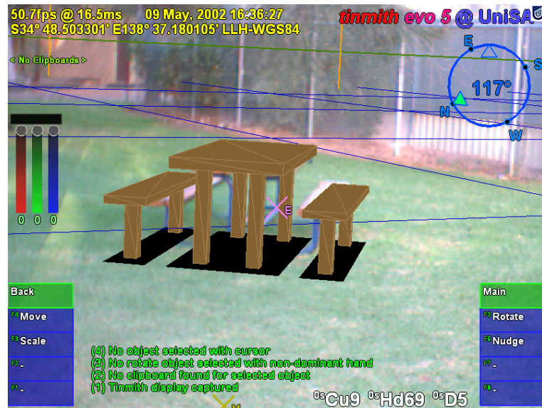
Figure 4-1 AR view of virtual table placed in alignment with physical world table
