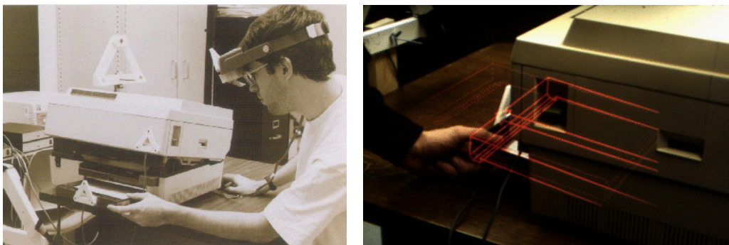
Figure 2-3 External and AR immersive views of a laser printer maintenance application (Images courtesy of Steven Feiner – Columbia University)
