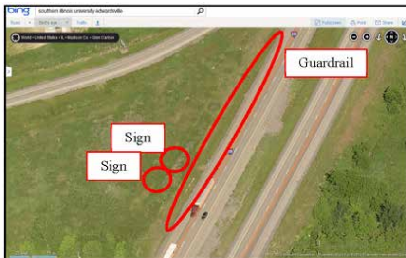
Figure 5-7. Data extracted by using satellite/aerial imagery method.
