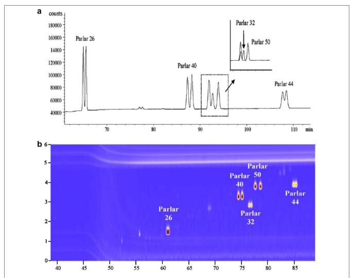
**Figure 3.** Enantiomer resolution of five toxaphenes by: (a) GC-ECD using a BGB-172 column; and, (b) GCxGC-μECD with BGB-172 × BPX-50 column combination. (Nomenclature: Parlar 26 = B8-1413; Parlar 32 = B7-515; Parlar 40 = B8-1414; Parlar 44 = B8-2229; and, Parlar 50 = B9-1679) (Reproduced from [29]).
