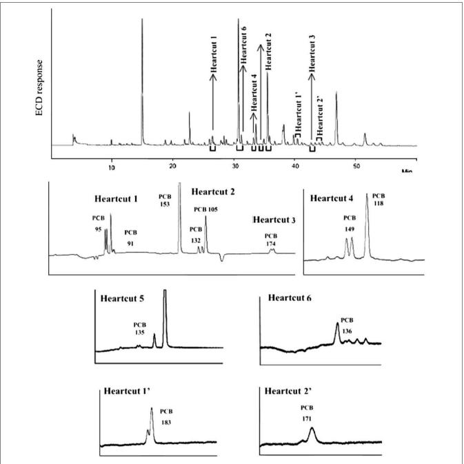
**Figure 2.** Chromatogram of a goat's milk sample and subsequent heart-cuts to Chirasil-Dex for the determination of congeners 91, 95, 132, 135, 149 and 174 (heart-cut 1 to heart-cut 6), and to BGB-172 for the determination of congeners 171 and 183 (heart-cut 1' and 2') (Reproduced from [26].
