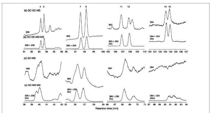
**Figure 4.** Chromatograms of a Swiss soil extract analyzed with: (a) heart-cut MDGC-MS<sup>2</sup>; (b) heart-cut MDGC-MS; (c) GC-MS<sup>2</sup>; and, (d) GC-MS. Monitored ions are indicated and magnification factors of MS<sup>2</sup> mass traces (a and c) are given in brackets. {Peak assignment: 4 = 95(E1); 5 = 95(E2); 7 = 149(-); 8 = 149(+); 11 = 132(-); 12 = 132(+); 14 = 174(+); and, 15 = 174(-) (Reproduced from [28]}.
