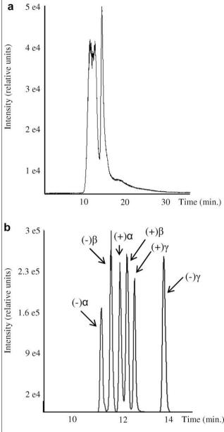
**Figure 5.** Chromatographic separation of HBCD standard mixture on: (a) ChiraDex column; and, (b) Nucleodex column.
