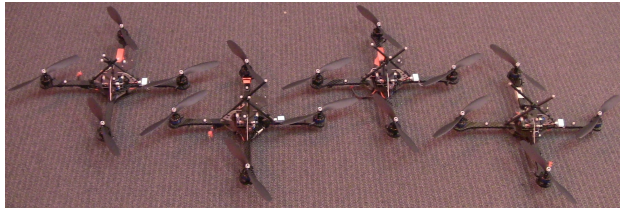
Fig. 3 The team of four quadrotors used in experimentation.
