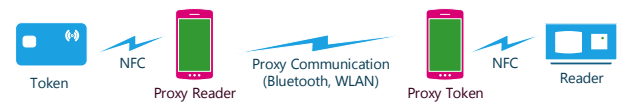
Figure 3: Schematic of a relay attack using a contactless smartcard, two NFC equipped phones and a reader terminal.
