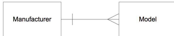
Figure 3-5 A crow's foot notation ERD indicating that one manufacturer makes many models
