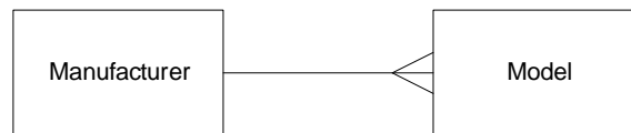
Figure 9-3 The standard relation FE in use – A manufacturer makes many models of car.
