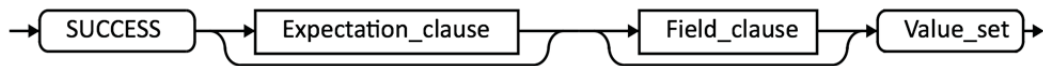
Figure F.15: Success answer with expectation and field clauses and a value set
