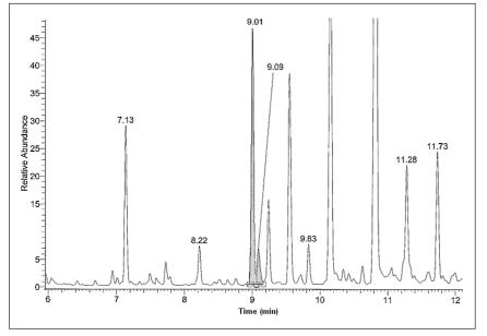
**Fig. 5a** Single quad GC/MS chromatogram (TIC) of an *Artemisia absinthium* L. extract (the unknown terpene at 9.01 min could be identified as linalool)
