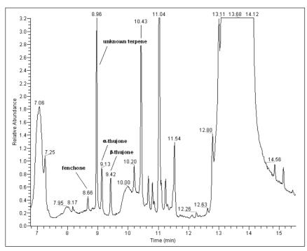
Fig. 3 GC/MS chromatogram (TIC) of sample 103, Versinthe Blanche ( $\alpha$ -thujone and the unknown terpene are present)
