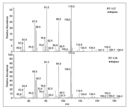
Fig. 4b Single quad mass spectra of  $\alpha\text{-}$  and  $\beta\text{-}thujone$
