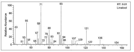
Fig. 5b Single quad mass spectrum of linalool
