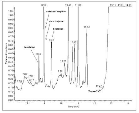
Fig. 2 GC/MS chromatogram (TIC) of sample 110, Candela (no  $\alpha$ -thujone, but another (first unknown) terpene and fenchone)
