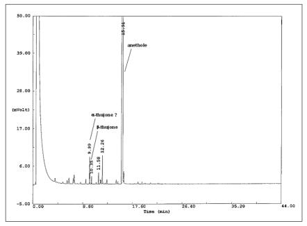
Fig. 1 GC/FID chromatogram of sample 110, Candela; it implies the presence of  $\alpha$ - and  $\beta$ -thujone
