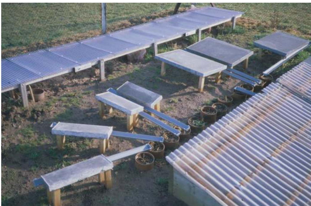
Plate 6-1 Biobed lysimeters subjected to a range of hydraulic loadings
