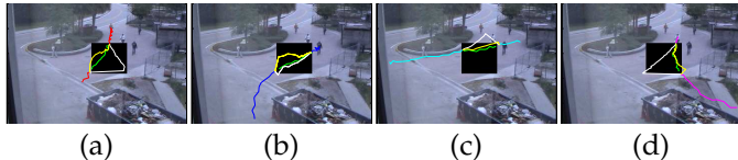
Fig. 15. Results for scenario shown in figure 14. Green track is the ground truth. Tracking through occlusion using Kalman filter is shown in white and yellow tracks are generated using the proposed approach. Notice that both methods can recover well once the measurement is available again, but during occlusion the proposed method stays closer to ground truth.
