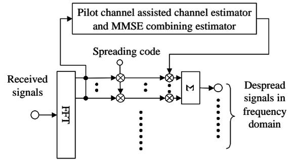
Fig. 5. Pilot channel assisted MMSE combining.
