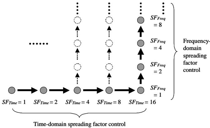
Fig. 4. Two-dimensional  $SF$  control in VSF-OFCDM.
