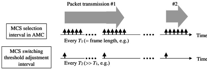
Fig. 3. Timing relation of adaptive radio link control.
