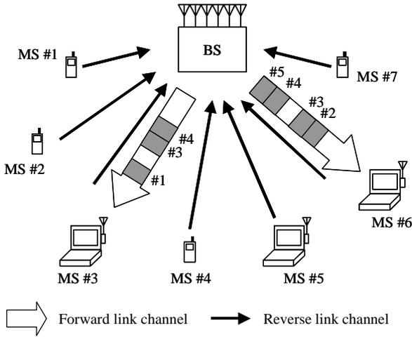
Fig. 6. Asymmetry between forward and reverse link channels.
