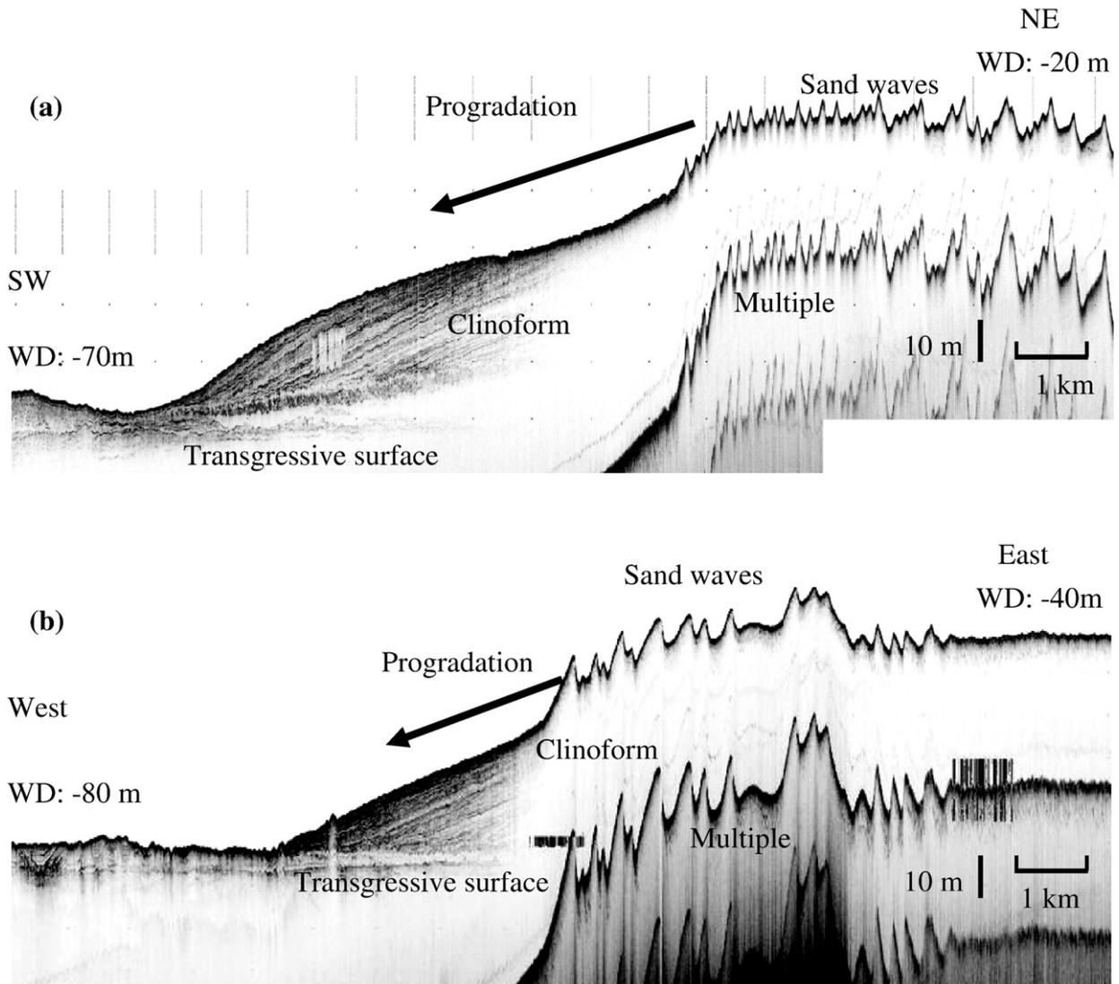
Fig. 6. Chirp sonar profiles in the central southern Taiwan Strait show a subaqueous delta progrades southwestward (a) and westward (b), and ends at water depth, -70 to -80 m off the Choshui River mouth. Topset of the cliniform is dominated by distinct sand waves, 2–5 m high.
