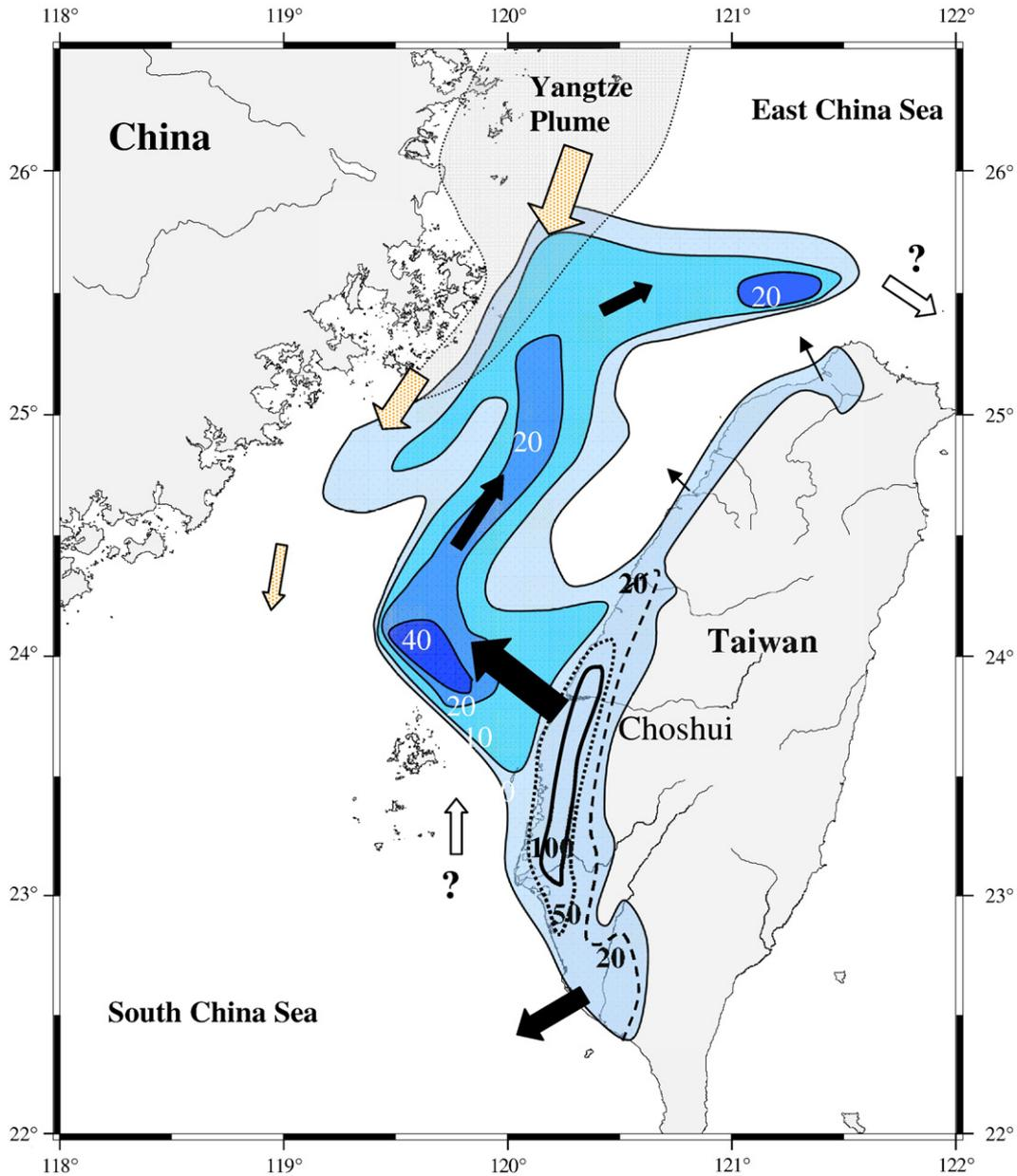
**Fig. 12.** Isopach of the post-glacial fluvial sediment distribution in the Taiwan Strait. The onshore part are made based on data from Cheng et al., 1999; Chen and Liu, 2003; Hsieh et al., 2006. The black arrows represent the inputs and transport of the Taiwanese rivers derived sediment to the strait. The open arrows with question mark (?) represent unknown transport. The shallow arrows represent the inputs from Yangtze and other mainland rivers.
