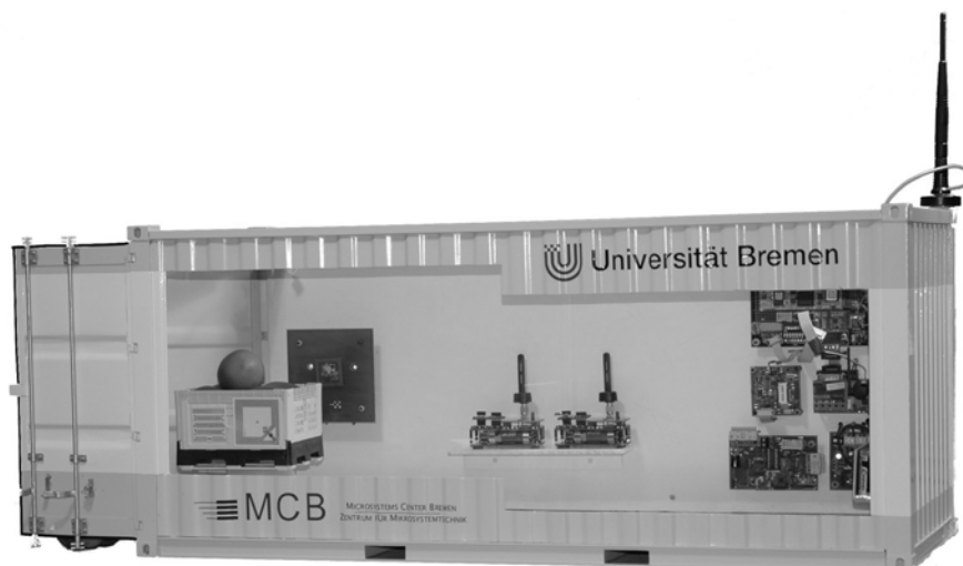
Fig.1. Reduced scale (1:8) prototype of the intelligent container. Loaded freight items are scanned by the RFID-Reader on left hand side. Sensor nodes supervise the environmental conditions (middle). A processor module on the right hand side executes a software agent containing specific transport instructions and quality modelling. The module for external mobile communication is placed on the right hand side panel.
