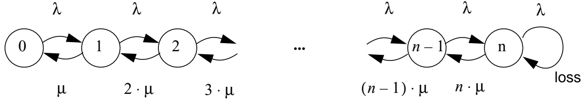
Figure 4.1: State transition diagram of a one-dimensional loss system
