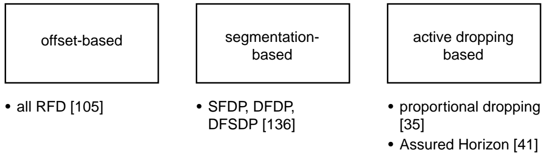
Figure 3.11: Classification of OBS-QoS mechanisms
