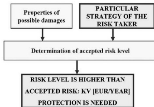
Figure 5.7.: Determining the need of protection – risk assessment component used in the SCOUT system (also used generally) [69]
