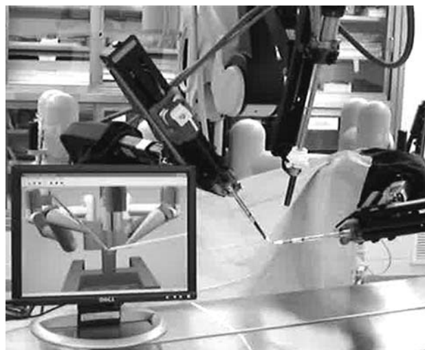
Fig. 3 The VR simulator ( left ) was constructed using the simulation software Webots (Cyberbotics Ltd., Lausanne, Switzerland). The da Vinci instruments and training task platform were modeled as 3D objects using SolidWorks (SolidWorks Corp., Concord, MA, USA). This simulation was driven by the kinematic data from the robotic operating console through LabVIEW (National Instruments, Austin, TX, USA)
