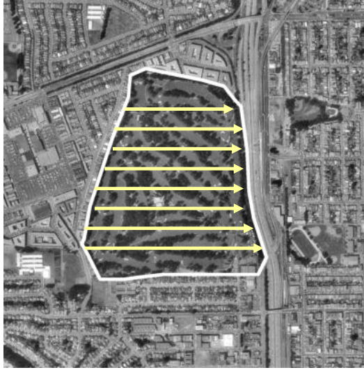
Figure 5.4: The arrows indicate different observation sequences sampled from an instance of a golf course at an angle 90^\circ w.r.t. the vertical. Sequences collected from several instances are used for estimating the parameters of the model \lambda(90^\circ, r) where r is the sampling step.
