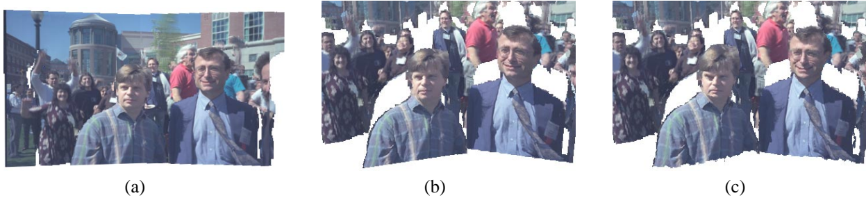
Figure 5: 3D views of the reconstructed symposium scene: (a) re-synthesized third image (note extended field of view). (b) novel view without residual depth; (c) novel view with residual depth (note the “rounding” of the people).
