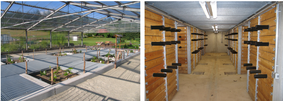
Figure 5. Aspects of the Göttingen Rhizolab Facility: containers aboveground covered by the mobile roof (left) and containers belowground with mini-rhizotron tubes (right).
