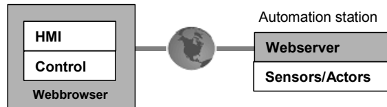
Fig. 5: LWA component structure for the telepresence lab
