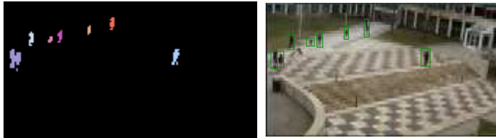
Fig. 2. Background mean image, blob segmentation image and input image with blob bounding boxes of Gaussian distributions at each pixel, as in Pfister [24]. However we finally opted for the eigenbackground method because it offered good results and less computational load.
