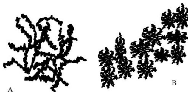
Fig. 2 A cartoon showing linear weakly cross-linked and highly branched clusters, A: acid catalyzed B: base catalyzed hydrolysis.
