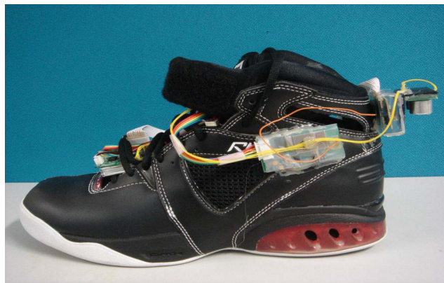
Figure 3.5.: Intelligent shoe proposed in [HCH07]
