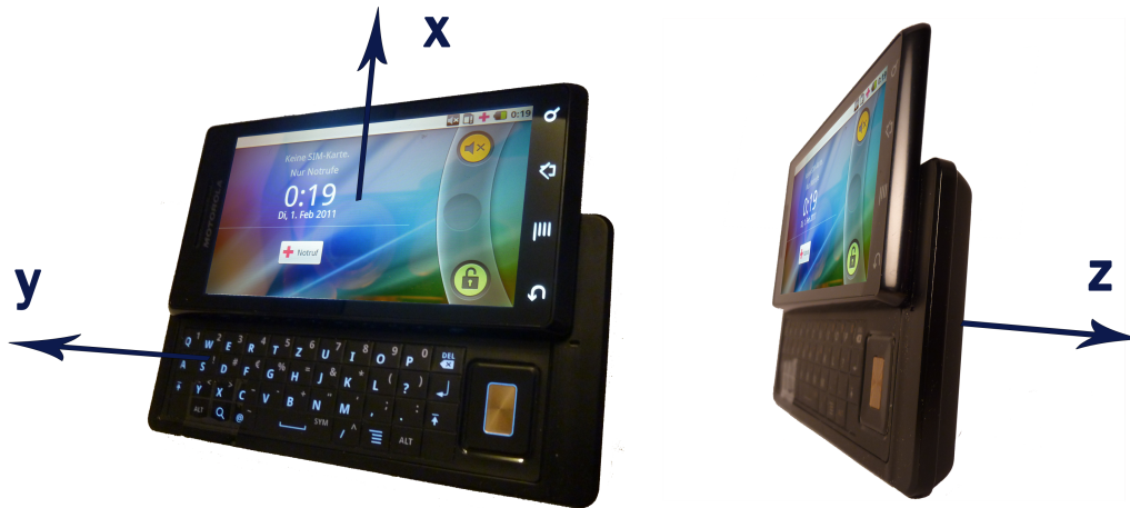
Figure 5.4.: Directions of the accelerometer dimensions
