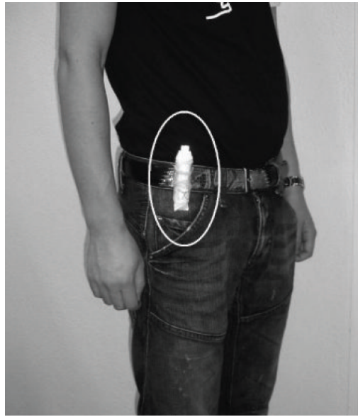
Figure 3.6.: Accelerometer placement on the hip in [GS09]
