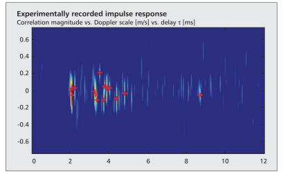
**Figure 5.** Example channel from the SPACE08 experiment, where correlation values  $\mathbf{A}^{H}\mathbf{z}$  are plotted in a grid according to their delay  $\tau_{q}$  and Doppler scale  $a_{p}$ : we make out about fifteen paths with a delay spread of maybe 10 ms and a Doppler spread of  $\sigma_{v} = 0.1 \text{ m/s}$ .
