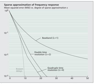
**Figure 2.** Comparison of MSE of sparse approximations of  $H(f_k)$  using s terms with various basis models; all cases lead to better approximation with larger s, but using a redundant basis leads to significantly fewer terms; the parameters are P = 10, K = 256.
