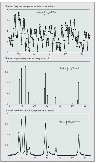
**Figure 1.** The channel frequency response H(f) maps to the impulse response  $h(\tau)$ , but from a limited number of samples  $H(f_k)$  only the baseband model  $h(\ell)$  can be determined unambiguously; in this example there are P = 10 discrete paths, and K = 256 frequency samples; all plots are magnitude only.
