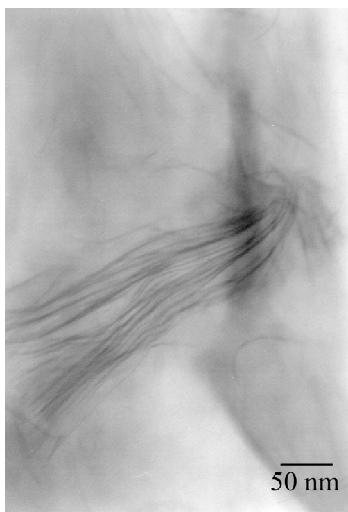
Fig. 5 TEM micrograph showing the peeling off layers from a silicate particle in a PP nanocomposite, changing gallery distance and varying extent of intercalation. Composition: 0.5 vol% silicate, 60 vol% MAPP.
