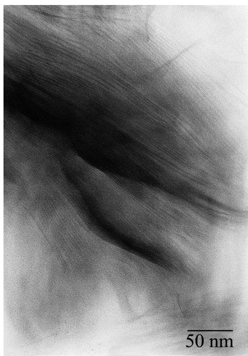
Fig. 4 TEM micrograph taken from a PP/OMMT/MAPP nanocomposite. Composition: 3 vol% silicate, 20 vol% MAPP.
