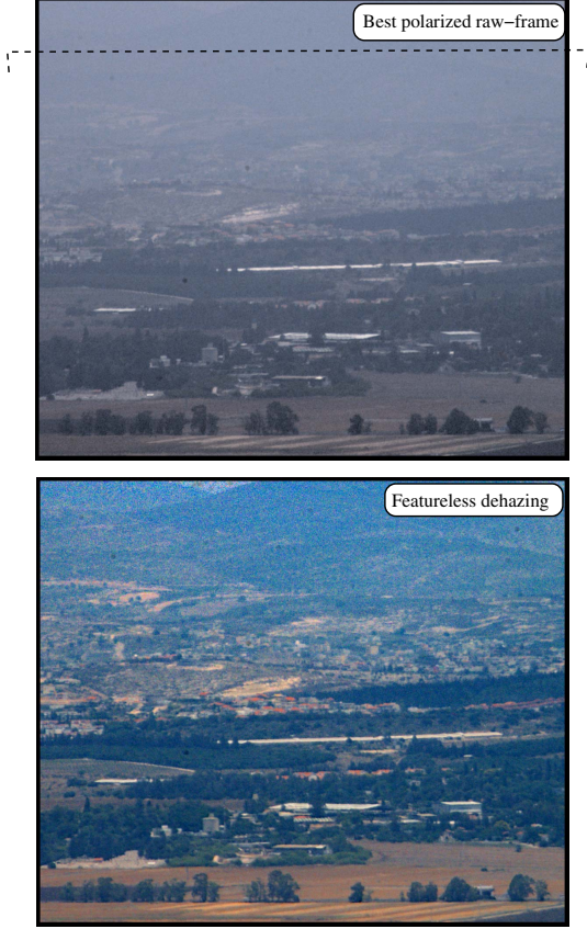
Figure 5. Featureless dehazing of Scene 2. The parameters \hat{p} and A_\infty were estimated using a cropped image reside below the dashed line
