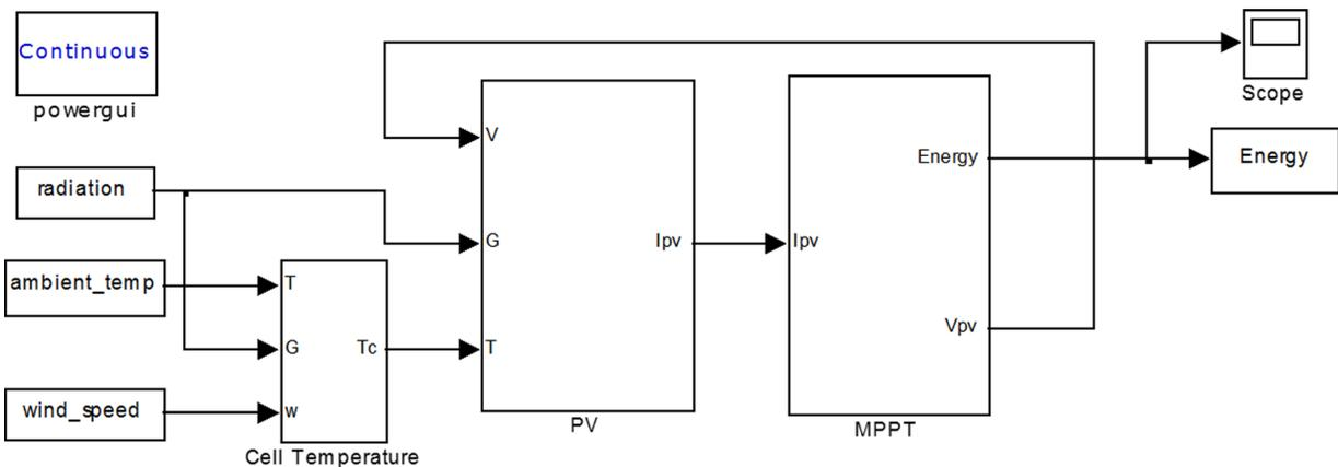
Fig. 5 MATLAB/SIMULINK block diagram of PV panel
