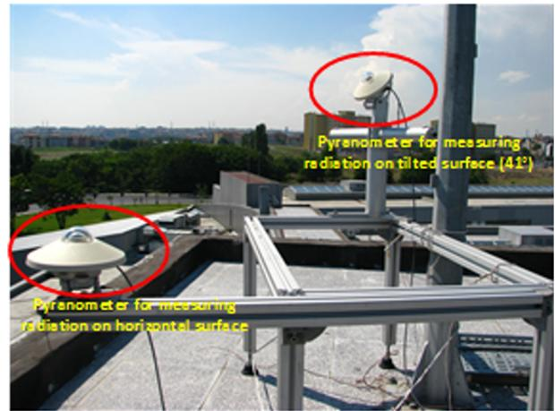
Fig. 2 Measurement setup for global radiation on horizontal and tilted surfaces
