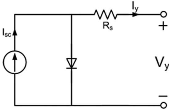
Fig. 4 Simplified equivalent circuit model
