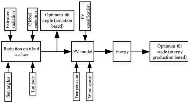
Fig. 1 The block diagram of the methodology
