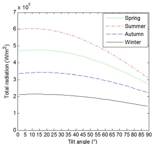
**Fig. 7** Total radiation on a square meter area for different tilted surfaces
