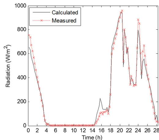
Fig. 3 Comparison of calculated and measured radiations on tilted surface
