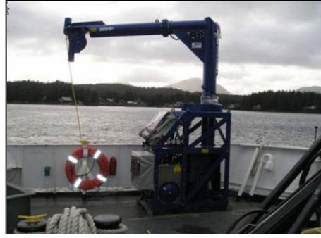
Figure 7. Moving vessel profiler mounted on fantail
