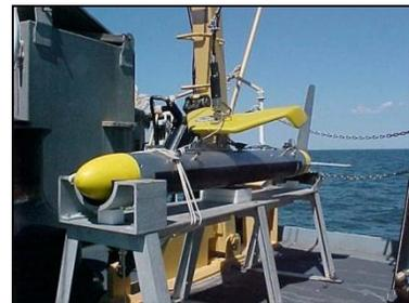
Figure 5. L-3 Klein 5000 side scan sonar
