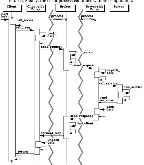
• When the client-side proxy receives the response, it unpacks the result and returns. Finally, the client process continues with its computation.
