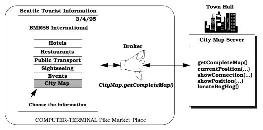
Since we expect the system to change and grow continuously, services should be decoupled from each other. In addition, the terminal software should be able to access services without knowing their location. This allows us to move, replicate, or migrate services.  $\Box$
