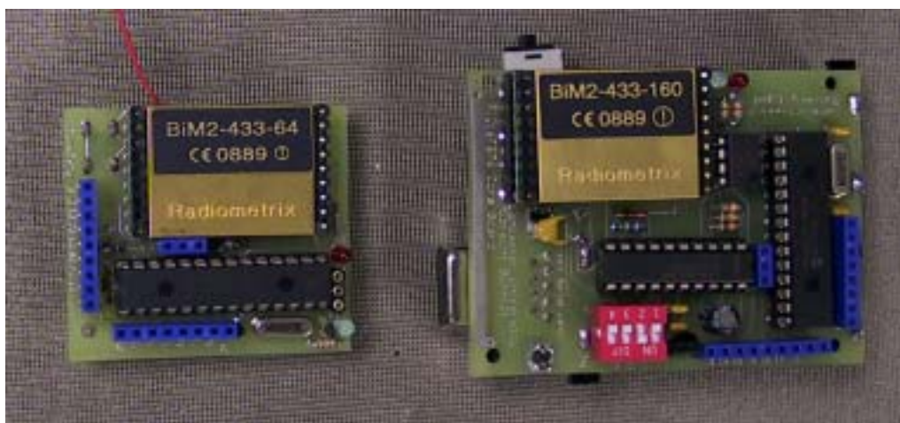
Figure 17: Smart-Its Core Boards.
