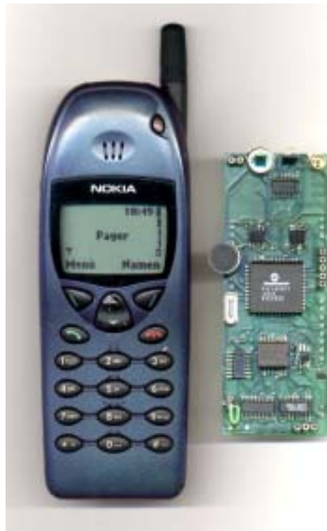
Figure 7: The sensor board and the enhanced mobile phone prototype.
