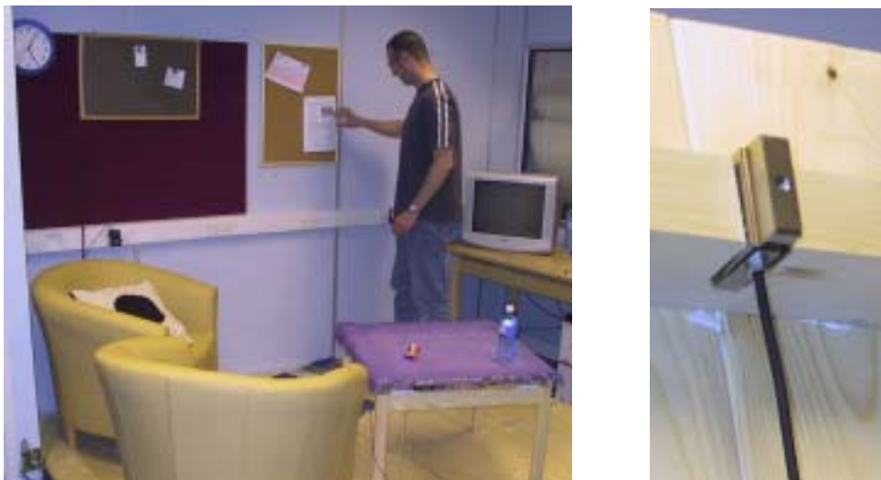
Figure 11: The floor installed in the lab setting (left). Enlarged view of the load cell embedded into the floor (right)
