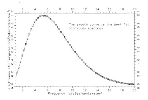
FIG 1: Fit of the measured cosmic background microwave radiation with Planck's equation for T = 2.735 K [13]. The first author, J.C. Mather, shared with his colleague G.F. Smoot the 2006 Nobel prize for physics.
