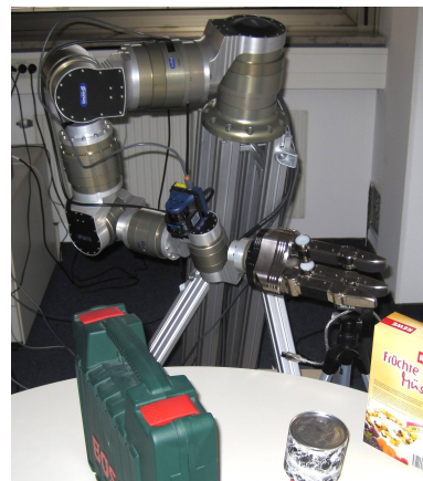
Fig. 8 The Schunk robot arm, the SDH hand and an arm-mounted Hokuyo URG-04LX laser.
