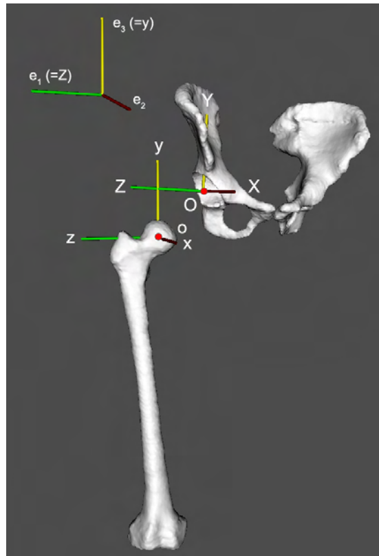
Figure 3.7: The pelvic coordinate system ( XYZ ), the femoral coordinate system ( xyz ), and the joint coordinate system ( e_1e_2e_3 ) for the right hip joint.
