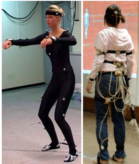
Figure 2.6: The two main motion capture systems: a) optical (Vicon) b) magnetic (Ascension).
