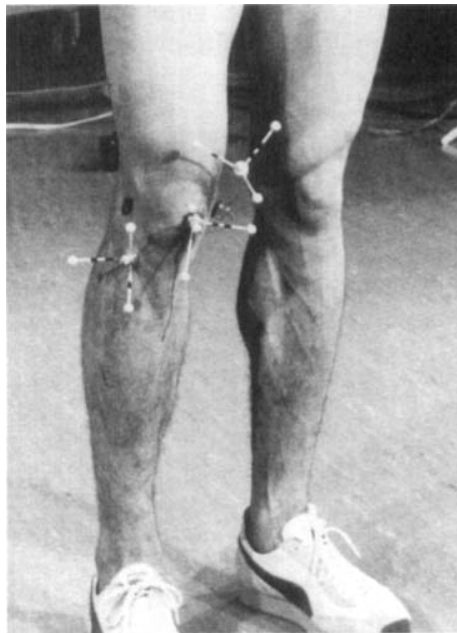
Figure 2.1: View of one subject with the triad targets attached to the tibial, femoral and patellar pins. Image from [LCS + 94] used by permission.
