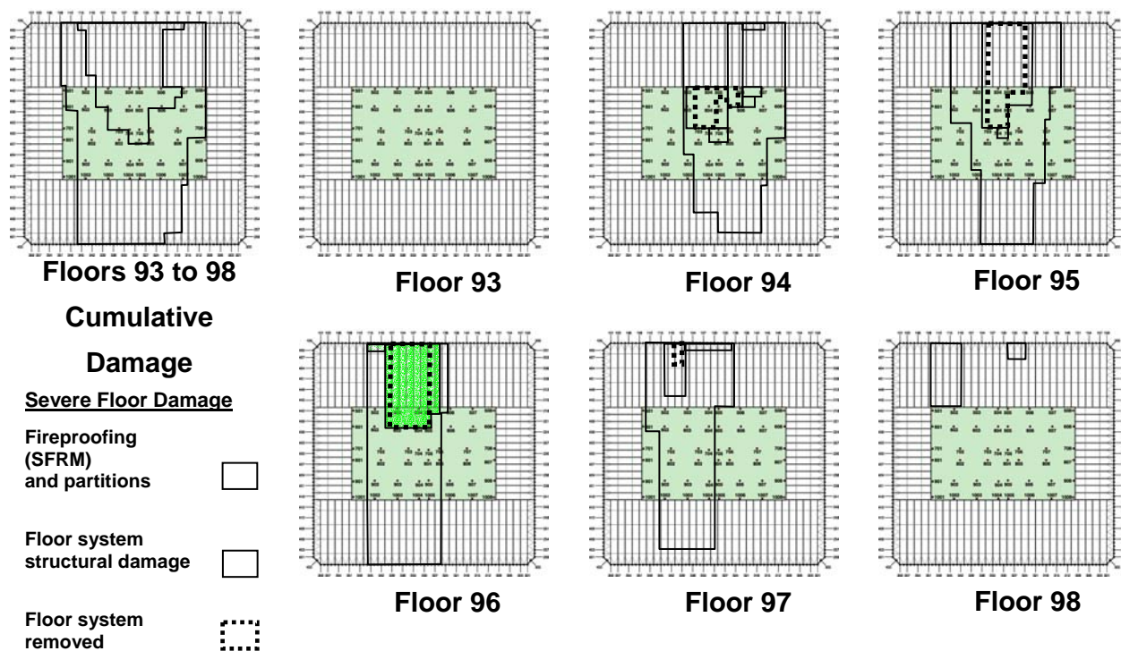
Figure 5-3. Calculated damage to floors 93 through 98 in WTC 1.
