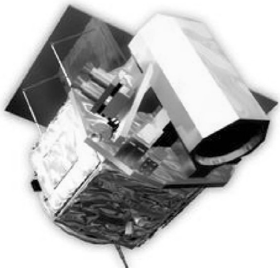
Fig. 2. The exterior view of the ROCSAT-2 and the layout of the ISUAL instrument. The hexagonal object on the top of the spacecraft is the telescope of the remote sensing imager, and the three instruments of the ISUAL payload is located at the left of the upper deck. From left to right, the instruments are a CCD imager, two array photometers and a 6-channel spectrophotometer.
