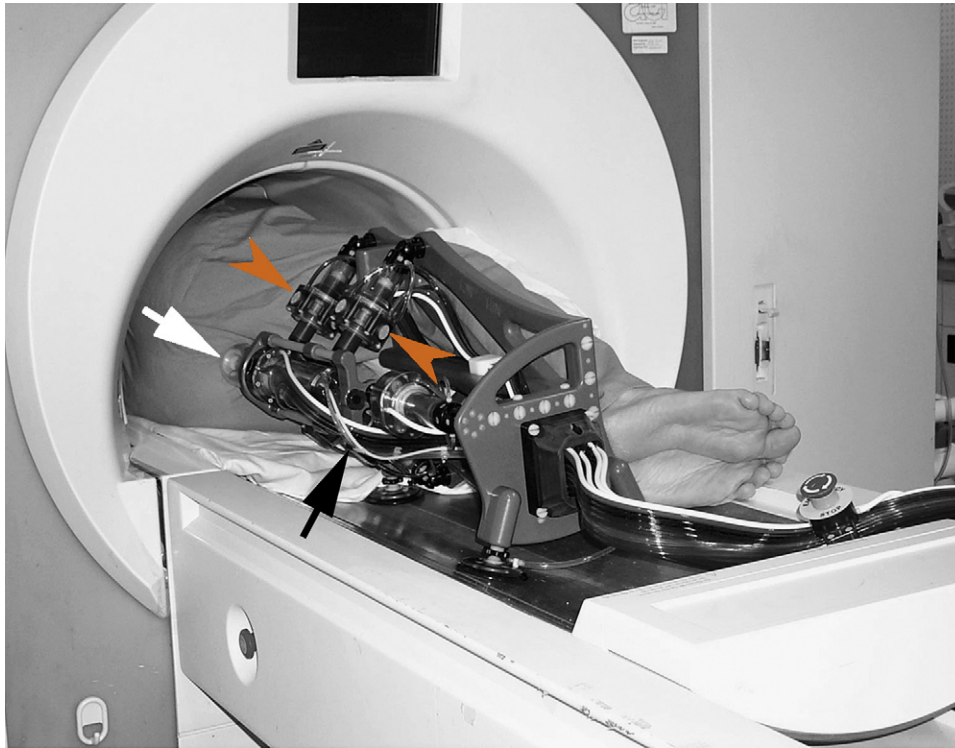
Fig. 4 – MrBot (black arrow) aligned with the patient in decubitus position. Pneumatic stepper motors (arrowheads) orient the end effector for transperineal intervention (white arrow) based on output from the guiding software. Courtesy of D. Stoianovici.
