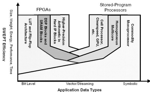
**Figure 1: FPGAs versus stored-program processors**
