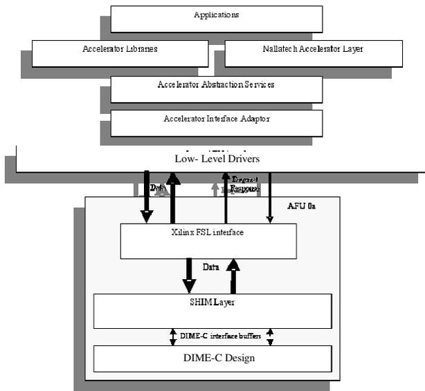
**Figure 5: System overview of an application using an FSB-FPGA accelerator module**
