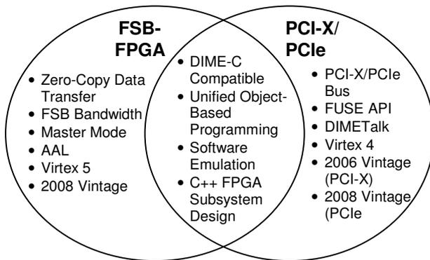
**Figure 4 – Comparison of FSB-FPGA and H101 platforms**
