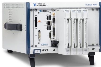
Figure 4: (a) example of an FPGA chip (source: XILINX). (b) PXI system (National Instruments) used as central control system for the LM-Q machine.
