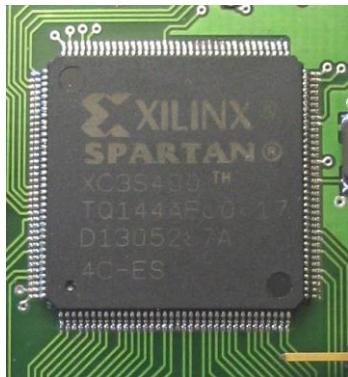
Figure 4: (a) example of an FPGA chip (source: XILINX). (b) PXI system (National Instruments) used as central control system for the LM-Q machine.
